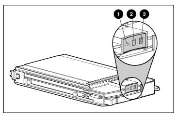
Figure E-3: Hot-plug SCSI hard drive LEDs
